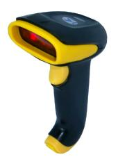
SL-8371 is a single-line, hand-held laser scanner. Equipped with Honeywell's patented CodeGate™ and CodeSense™ technology.SL-8371can be used In a wide variety of applications. CodeSense™ technology allows the user to easily target the desired bar code and complete data transmission with the press of a single button. This makes SL-8371 a perfect selection for menu scanning, point -of-sale, document processing and inventory control.
